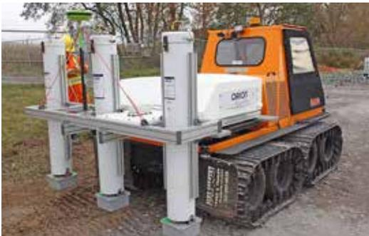
**Track-mounted vehicles equipped with ScanPlot technology are used to scan remediated areas of the legacy waste management facility for gamma radiation. The units capture GPS locations of any areas where gamma readings are detected. The results provides an indication if remediation has been completed in specific portions of the site or if further excavation is required to meet PHAI Clean-up Criteria.**
