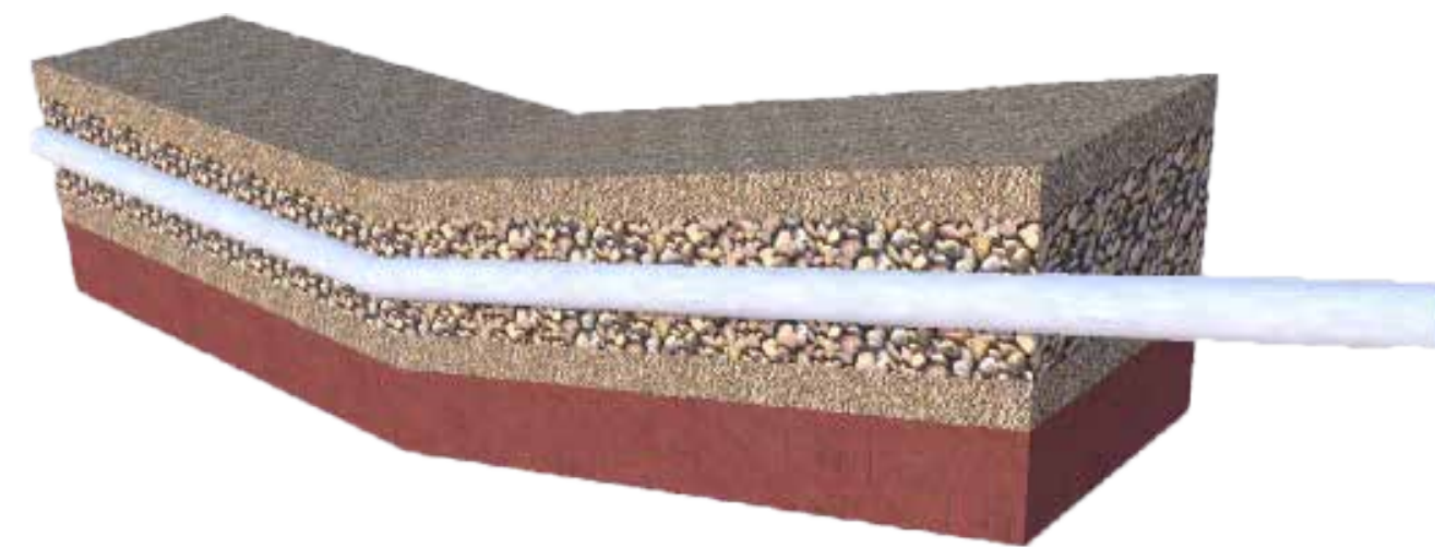
Leachate pumped from within the aboveground mound
