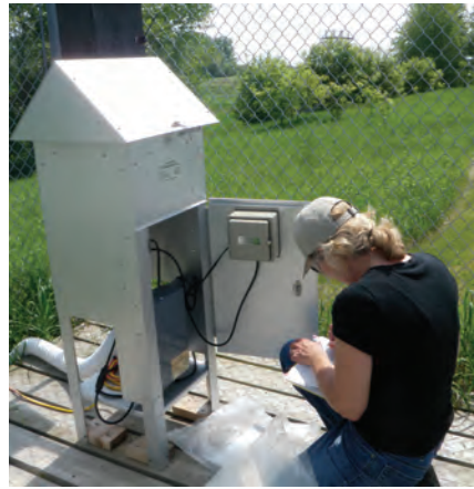
Technician changing filter in high-volume air sampler
