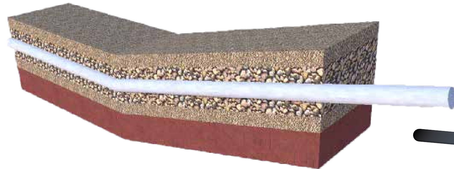
Leachate pumped from within the aboveground mound
