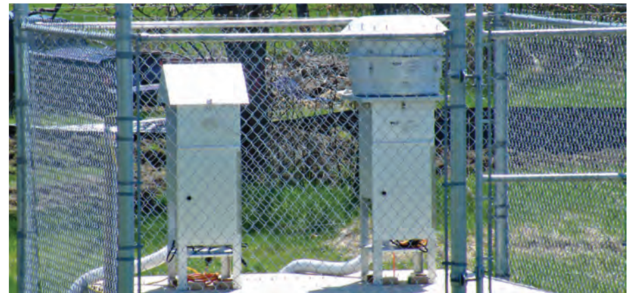
Fixed high-volume air samplers monitor air quality continuously
