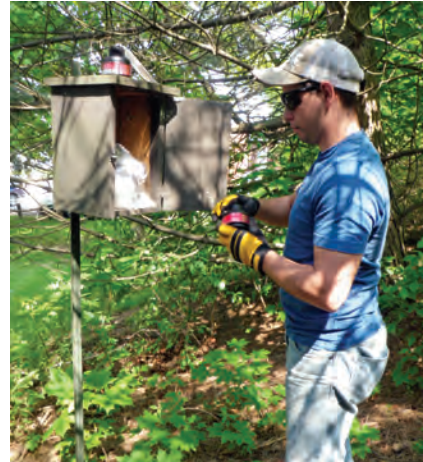
Monitoring air quality with high-volume air and radon samplers
